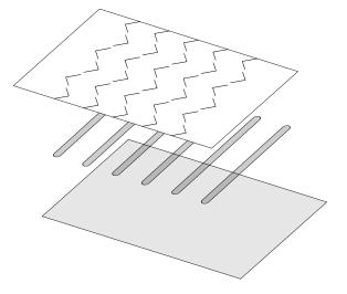
At a fundamental level, the 'pop-up' or shape-changing behavior occurs due to the differential compressive forces on the two layers. The pre-strained elastic substrate forces the thin, deformable top layer to buckle. Selective attachment of the top and bottom layers in the pre-programmed rows limits the buckling to localized rows of material.
